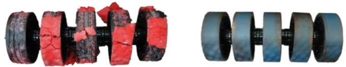
The hydrolysis-resistant tires can more than double the service life of running surfaces in comparison with conventional materials.
